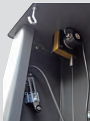
Height Limit Switch and Displacement Sensor
