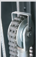
Chain support with derailment protection
