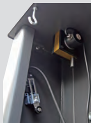
Height Limit Switch and Displacement Sensor
