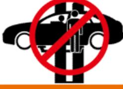
**Do not climb onto the lift or raised vehicle during lifting or lowering.**
