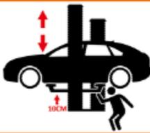
**Stop and check lift arm locks and stability of vehicle after short raising, then to desired height.**
