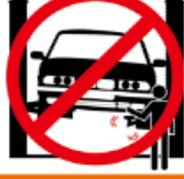
**Avoid excessive rocking of vehicle while on lift.**
