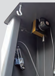
Height Limit Switch and Displacement Sensor
