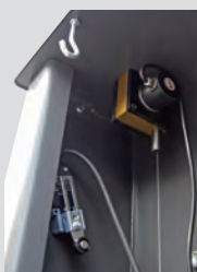
Height Limit Switch and Displacement Sensor
