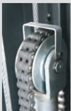
Chain support with derailment protection
