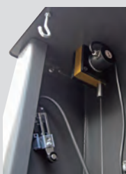
Height Limit Switch and Displacement Sensor
